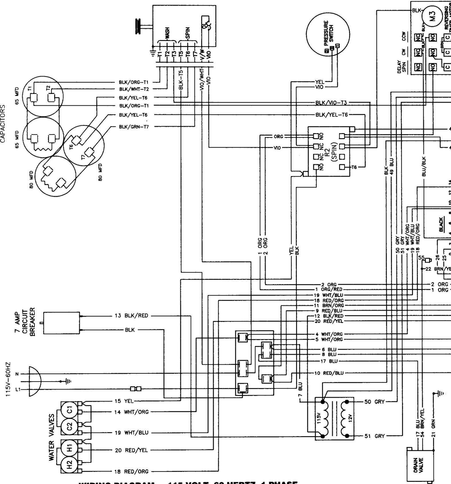
**WIRING DIAGRAM — 115 VOLT, 60 HERTZ, 1 PHASE**
